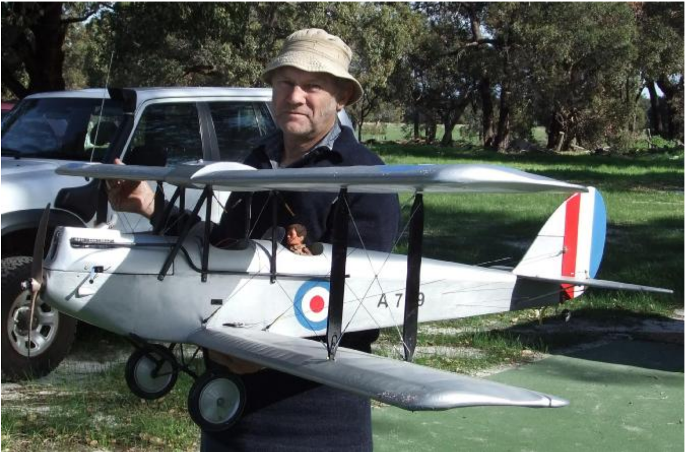
Dennis Buckland and Gypsy Moth. Powered by an OS 70 4st, and a very realistic flyer. Covered with Stig Coverall, an excellent and cost effective heatshrink woven material.
